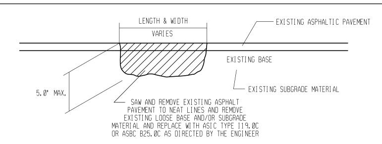
\*NOTE: EDGES OF PATCHED AREA ARE TO BE CLEANED OF ALL DEBRIS AND COATED WITH AN APPROVED TACK MATERIAL BEFORE PLACING ASPHALT.
